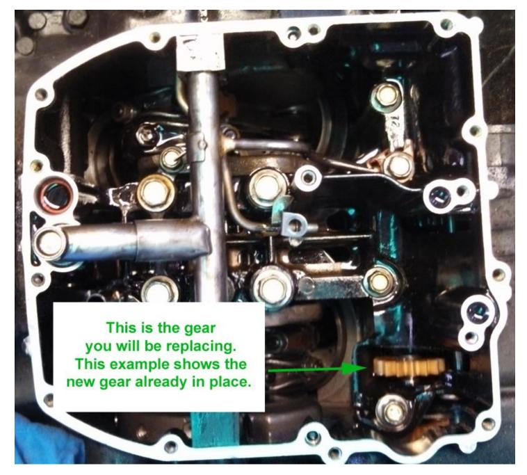
In the picture above, the oil pump has been removed and you can see the gear that you will need to replace. This engine already has a new gear in it. The particular gear is excellent condition used so it has turned a bit orange due to immersion in normally hot engine oil. Your gear may be white. It will be identical to the gear outside the case that engages the drive gear on the back of the clutch basket. The gear you remove will be slightly smaller.
