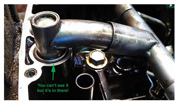
The photo above shows the oil distribution manifold re installed. Be sure to put the rubber bumper back on top of the tube the o-ring is sealing...or it won't seal anything. That bumper pushes against the oil pan when it is re installed and keeps the entire pipe from blowing out.
