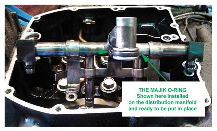
The photo above shows the oil distribution manifold removed, the old o-ring removed, and the oval cross section black Kawasaki o-ring installed. This one won't blow but be sure to oil it well before attempting to install it. Also make sure that the end of the pipe that it will be installed over is completely free of burrs so that it won't be scratched...or worse...cut. Carefully re-install the oil distribution manifold.
