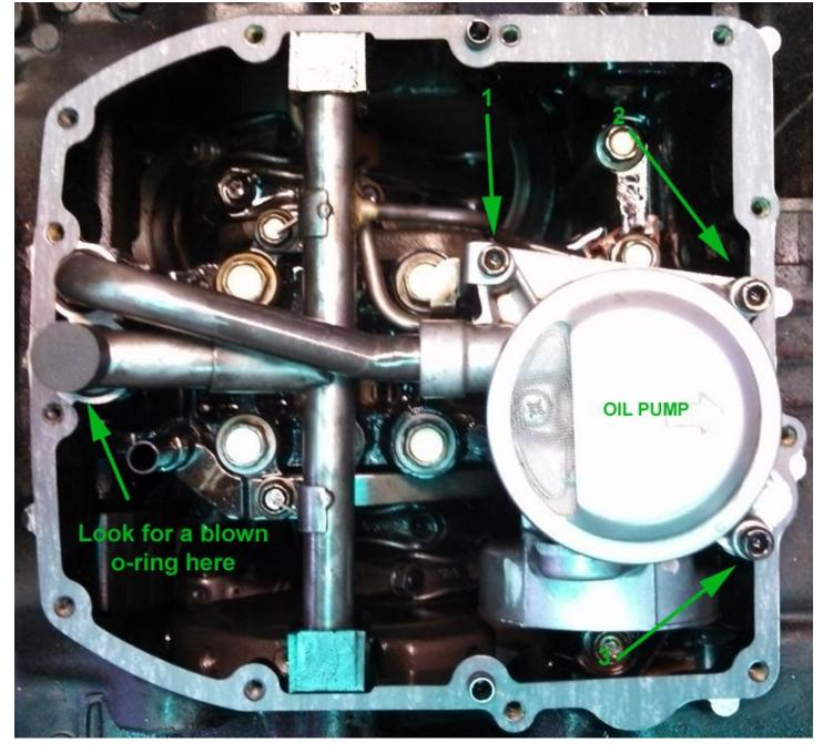
The picture above shows what you will see when the oil pan is removed. Note the arrow that points to where the o-ring that sometimes blows out is located. It will usually be bright orange. The other three arrows point to the three metric Allen bolts that retain the oil pump. Remove the oil pump and all its associated plumbing now.
