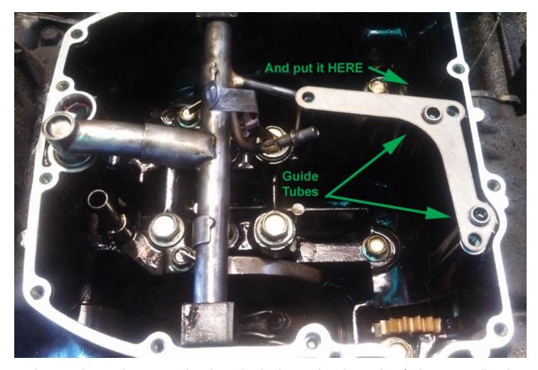
Put the spacer here as shown. Note the tube guides that keep it aligned properly to facilitate re-installing the oil pump assembly. And now you should re-install the oil pump assembly. Do not over tighten Allen screws. Some blue lock-tite might not hurt if you can de grease the bolt holes and the bolts without removing too much oil from around the area. Be sure to get all the pipes in the right place.
